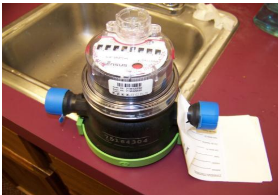
Left is a picture of a standard residential mechanical water meter located inside the house, on the right is an ERT (Encoder Receiver Transmitter) which will be mounted on or near the meter. Wires are used to connect the meter to the ERT which allows us to read the meter without entering your home.
