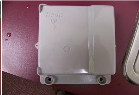
Left is a picture of a standard residential mechanical water meter located inside the house, on the right is an ERT (Encoder Receiver Transmitter) which will be mounted on or near the meter. Wires are used to connect the meter to the ERT which allows us to read the meter without entering your home.
